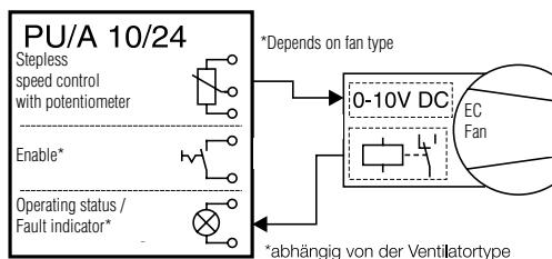
For the stepless control or regulation of one and three phase EC fans with a setpoint input of 0–10 V DC. Connection examples can be found in the basic circuit diagrams below.
